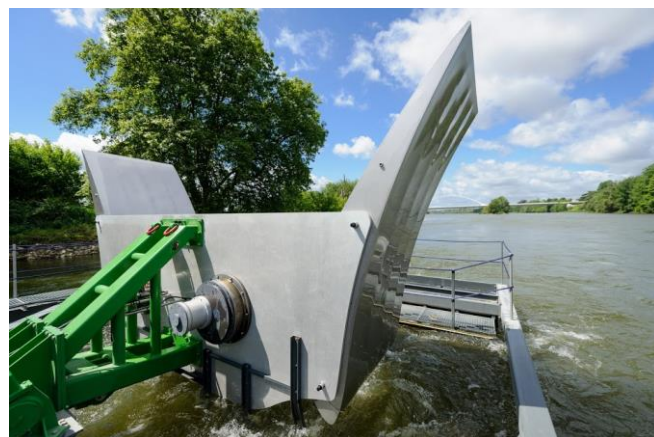
Figure 11. Picture of the hydrokinetic turbine, raised on the barge, in the river Loire at Orléans.
